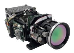
**TC640SMW** is a small-sized mid-wave cooled thermal imaging core with high-resolution detector which can be easily integrated into infrared systems that require extremly long distance detection and adaption to any harsh environment.
